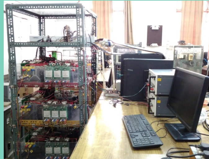
Prototype of high-resolution level doubling network based multi-level inverter
